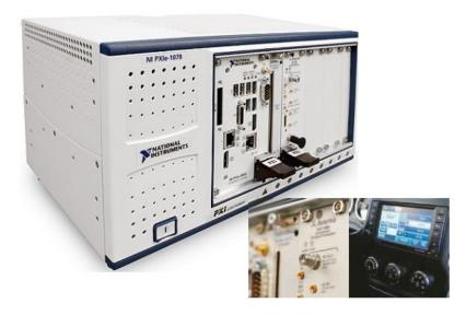
The National Instruments PXI platform is ideal because of the modular hardware platform that can be reconfigured with key software tools. For example, the same vector signal generator from National Instruments can be used to simulate GPS signals and can then be re-programmed to broadcast and simulate digital video broadcast, or DAB.
