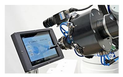
Our infotainment HMI testing is customized and the complete testing is automated using NI LabVIEW and TestStand software platform.
